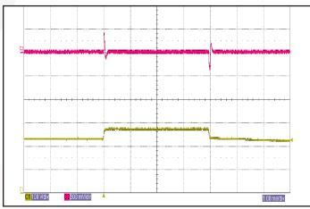
**Figure 12:** Output voltage response to step-change in input voltage (250V/ms). Load cap: 100  $\mu$ F electrolytic output capacitance. Ch 1: Vin (100V/div), Ch 2: Vout (500mV/div).
