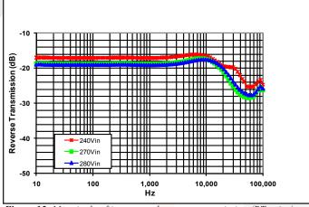
Figure 15: Magnitude of incremental reverse transmission ( $RT = i_{in}/i_{in}$ iout) for minimum, nominal, and maximum input voltage at full rated power.
