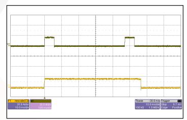
Figure 18: Load current (20A/div) as a function of time (10ms/div and 100ms/ div) when the converter attempts to turn on into a 10 m $\Omega$  short circuit.
