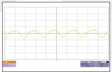
**Figure 9:** Input terminal current ripple,  $i_C$ , at full rated output current and nominal input voltage with  $100\mu$ H source impedance and  $47\mu$ F electrolytic Capacitor (200 mA/div). Bandwidth: 20MHz. See Figure 17.
