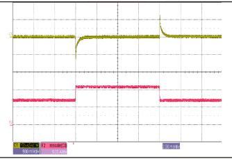
**Figure 11:** Output voltage response to step-change in load current (50%-75%-50% of lout(max);  $dI/dt = 0.1 A/\mu s$ ). Load cap: 1  $\mu$ F ceramic and 15  $\mu$ F tantalum capacitors. Ch 1: Vout (500mV/div), Ch 2: lout (5A/div).
