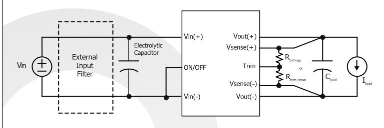
Figure D: Typical application circuit (negative logic unit, permanently enabled).
