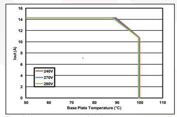
Figure 5: Maximum output current vs. base plate temperature .
