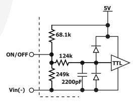
Figure B: Internal ON/OFF pin circuitry
