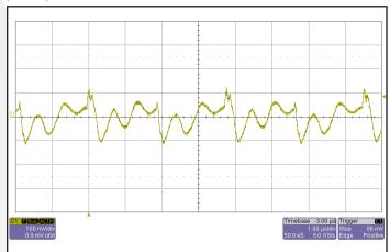
**Figure 10:** Output voltage ripple, Vout, at nominal input voltage and rated load current (100 mV/div). Load capacitance:  $1\mu F$  ceramic capacitor and  $10\mu F$  tantalum capacitor. Bandwidth: 10 MHz. See Figure 17.
